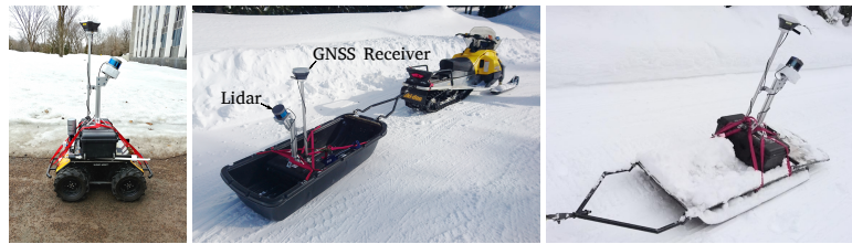
Fig. 5: Left : Rack mounted on a small robot for easy terrain (e.g. parking lot, sidewalks). Middle : Rack pulled by a snowmobile for maps on harden snow. Right : In last resort, the rack could be pulled by humans, which has proven to be useful on narrow/dense paths in the forest.
