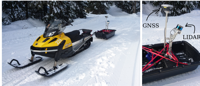
Fig. 2: The data acquisition platform mounted on a sleigh behind the snowmobile ( left ). This configuration limited transfer of engine vibrations to the sensors. Right : close-up of the GNSS receiver and the RS-16 lidar.
