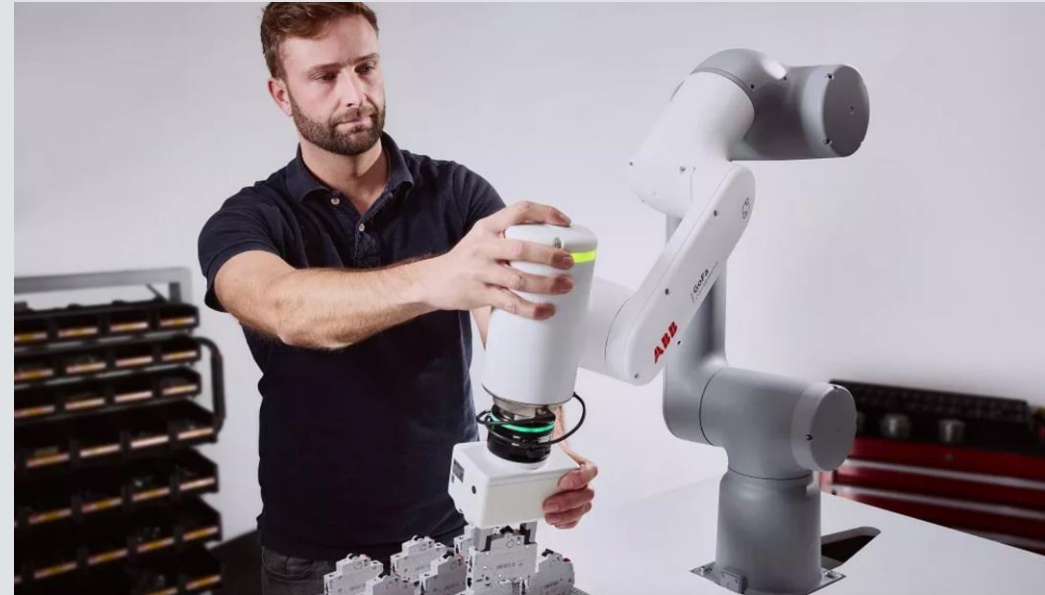
Fig. 1: Exemple de coopération physique humain-robot. ABB's GoFa cobot welding cell helps workers with repetitive, challenging tasks [image]. (2022, 1er décembre). The FABRICATOR. https://www.thefabricator.com/thefabricator/product/automationrobotics/abbs-gofa-cobot-welding-cell-helps-workers-with-repetitive-challenging-tasks
