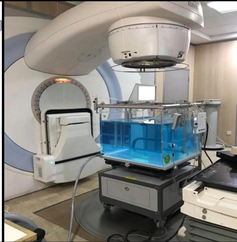
Measuring percentage depth dose of a ionizing radiation by a water phantom
